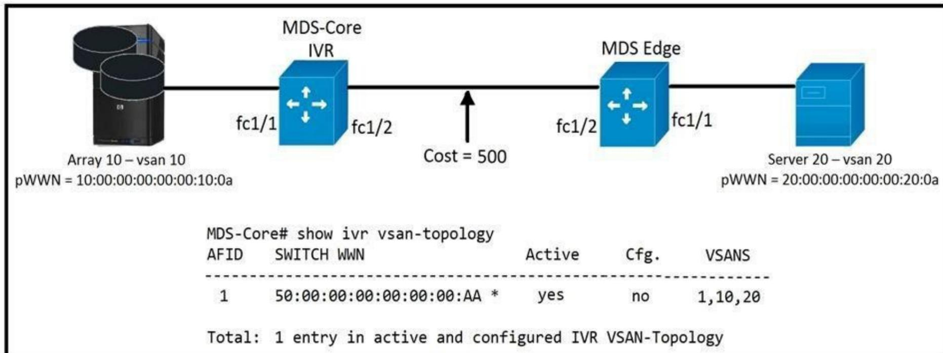
An engineer is configuring Inter-VSAN routing for two Cisco MDS switches. The FSPF cost between the switches is 500, and the Cisco MDS core virtualizes an IVR NAT domain as shown. Which statement about the topology is correct?
