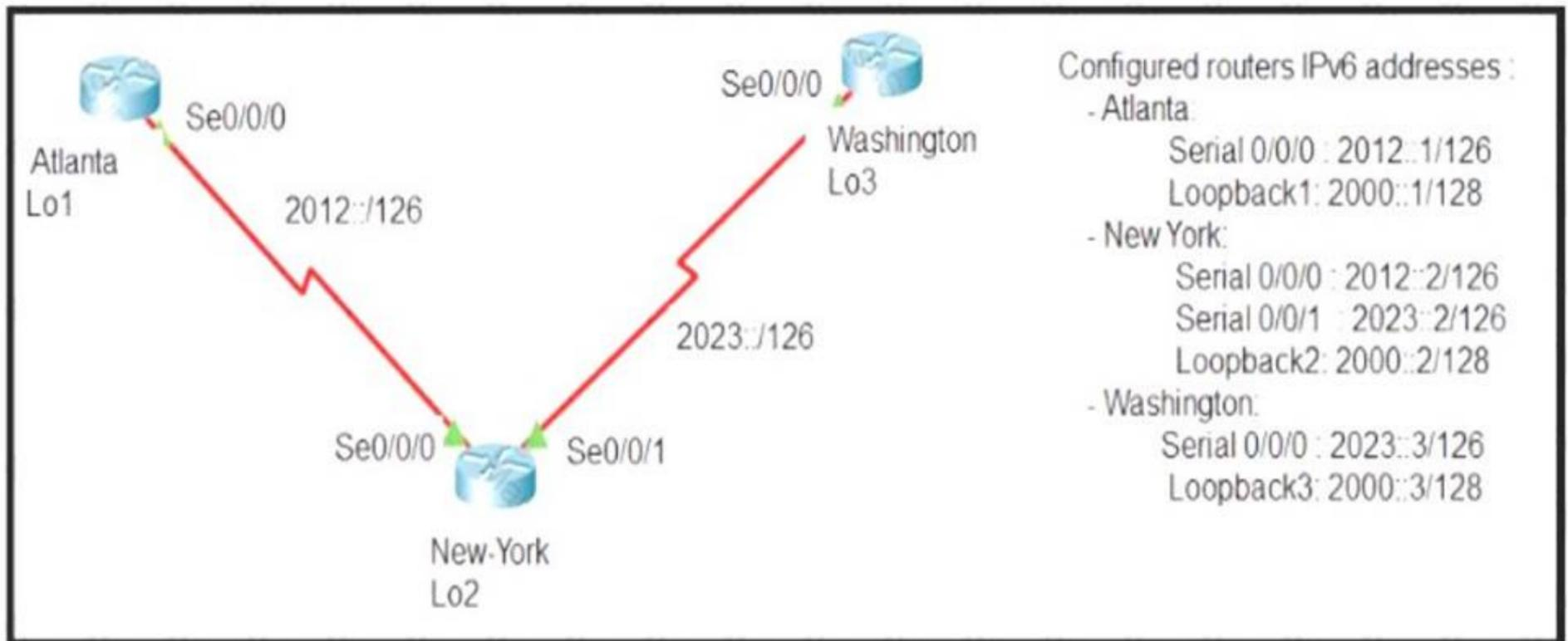
The New York router is configured with static routes pointing to the Atlanta and Washington sites. Which two tasks must be performed so that the Serial0/0/0 interfaces on the Atlanta and Washington routers can reach one another? (Choose two.)
