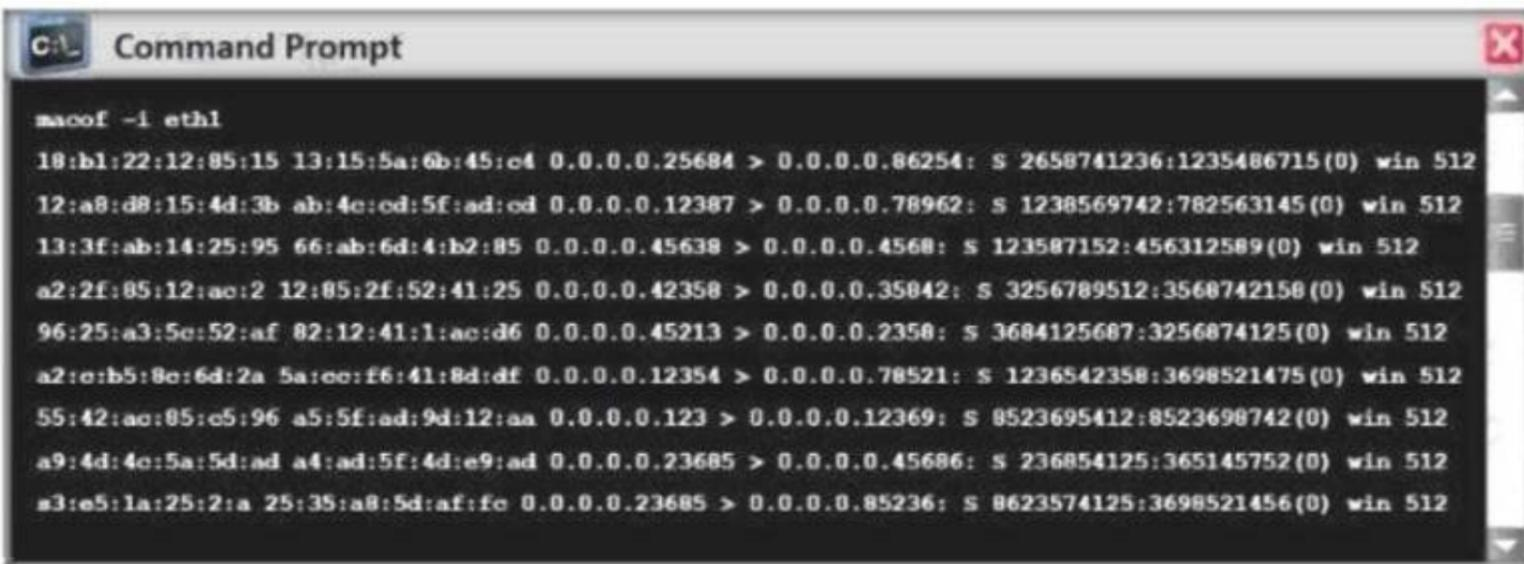
In MAC flooding attack, a switch is fed with many Ethernet frames, each containing different source MAC addresses, by the attacker. Switches have a limited memory for mapping various MAC addresses to physical ports. What happens when the CAM table becomes full?
