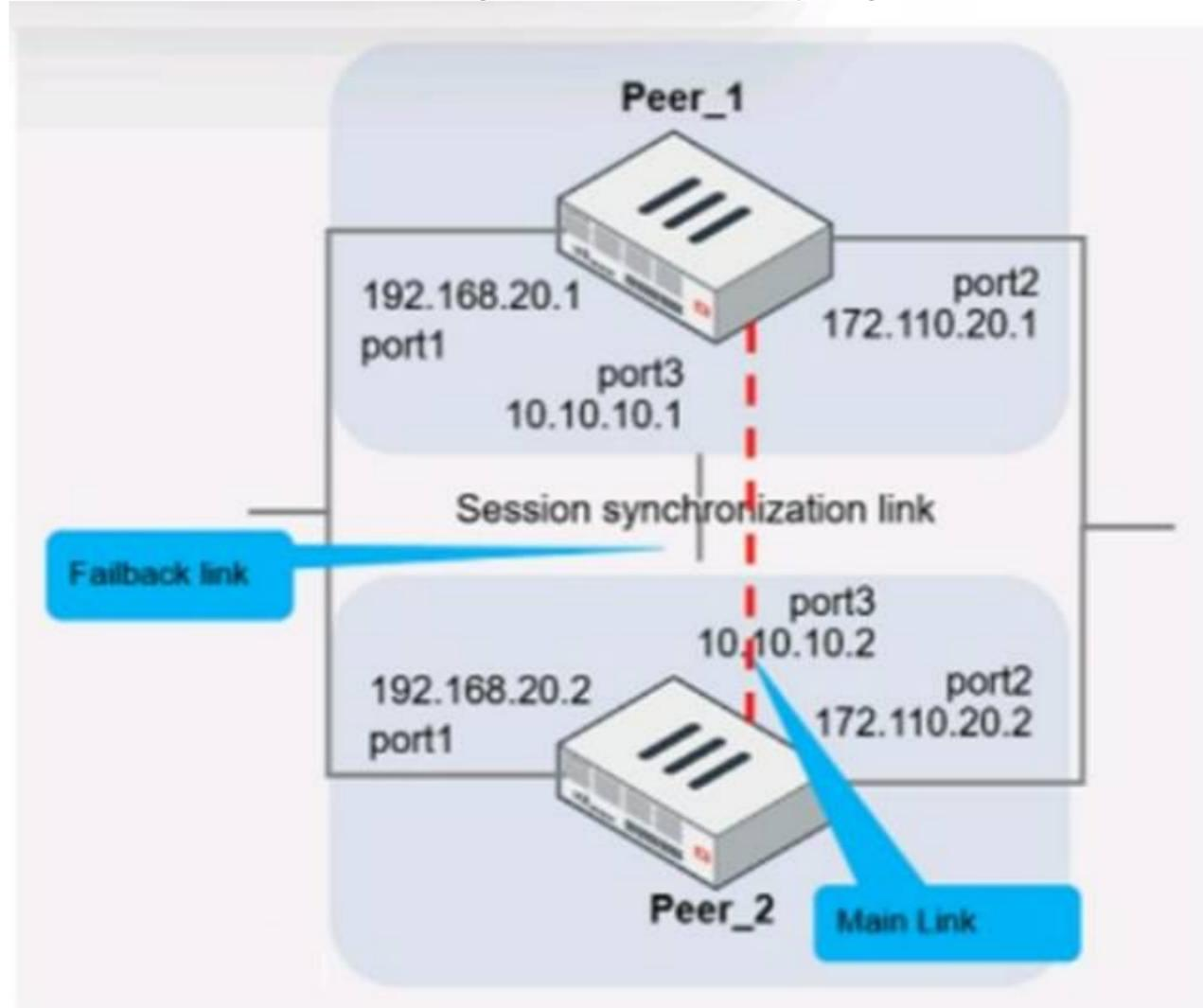
The main link directly connects the two FortiGate devices and is configured using the set session-syn-dev <interface> command.
