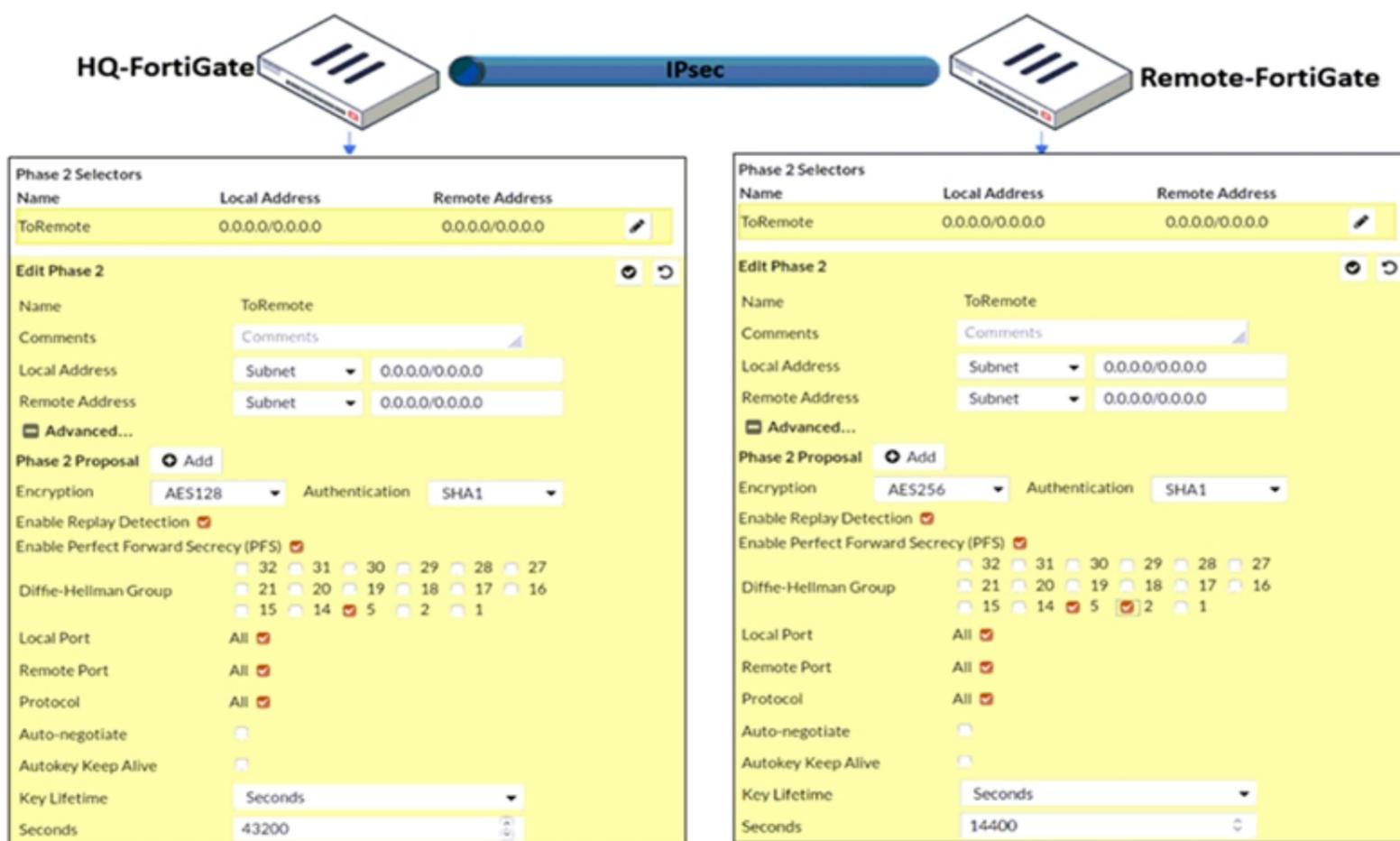
A network administrator is troubleshooting an IPsec tunnel between two FortiGate devices. The administrator has determined that phase 1 status is up. but phase 2 fails to come up.
